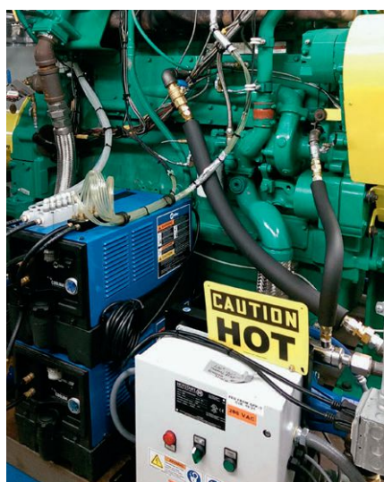
Cummins QSK19G natural gas engine (for power generation, not autos); Argonne Engine Test Cell. The Advanced Laser Ignition System (ALIS) was used on the Cummins natural gas engine to demonstrate better efficiency than stock ignition systems. (Courtesy of Argonne National Laboratory)
